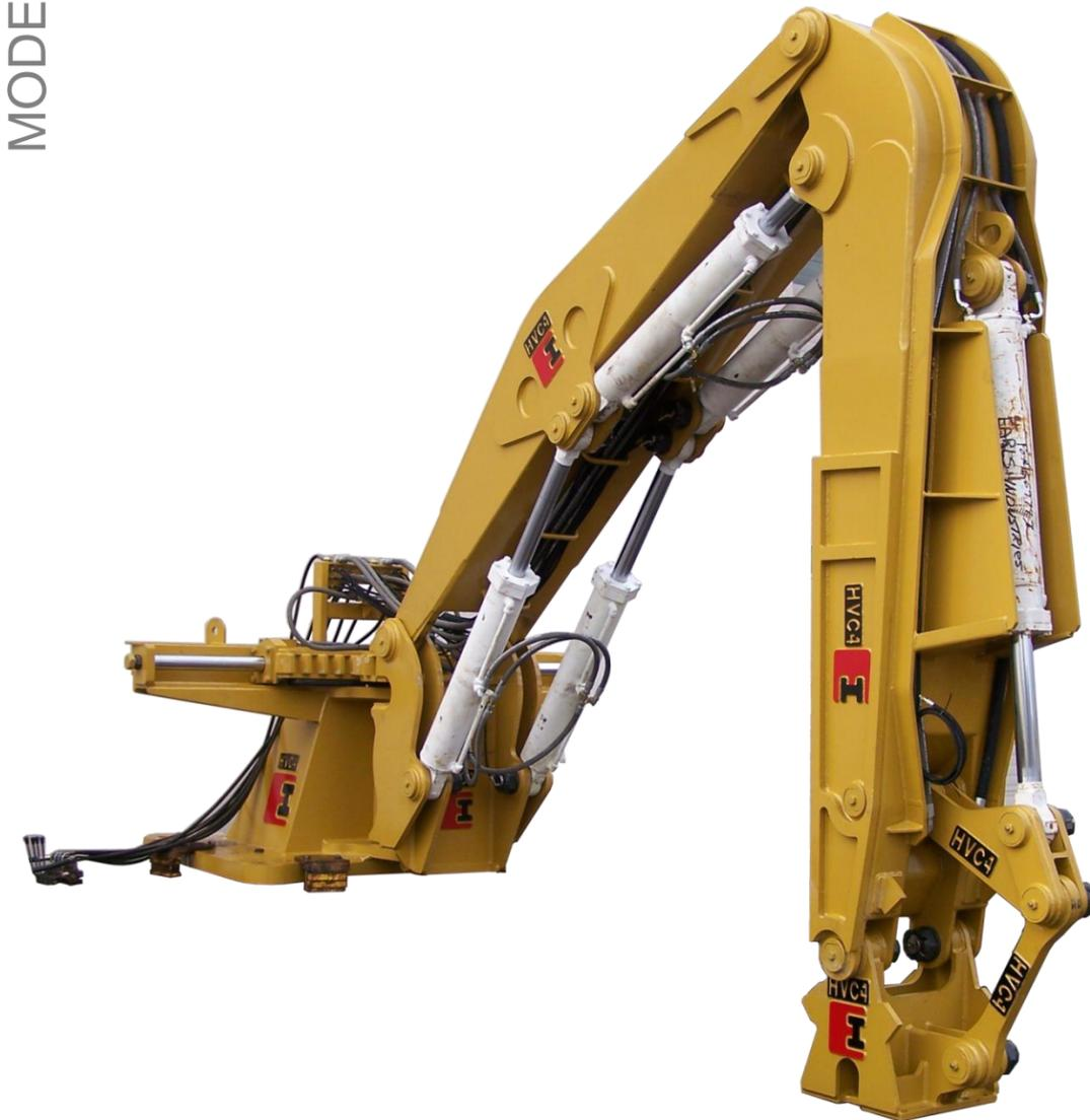
The EARLS rock breaker boom is a high strength articulating structure designed to manipulate hydraulic breaker hammers, rock grapples, and rock points. It consists of the following major components; base mount, boom foot swivel, boom, stick and tool mount.
